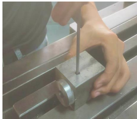
4. Lock the set screw of the barrel.
