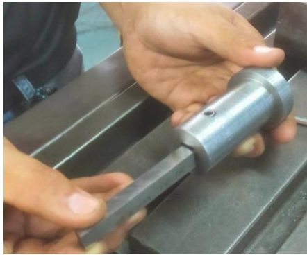
1. Place the tool blank inside the sleeve.
