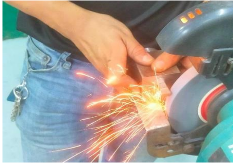
9. Grind the side relief using the tool bit jig.
