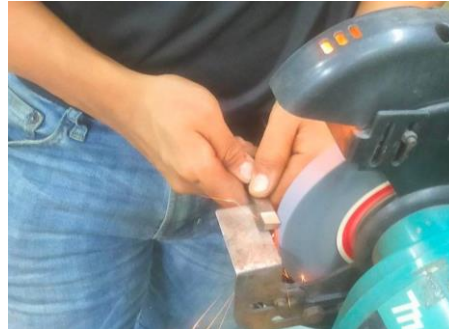
10. Grind the side relief using bare hands.
