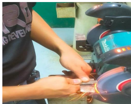
6. Grind the end relief angle using bare hands.
