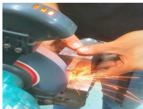
7. Grind the side rake using the tool bit jig.
