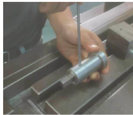
2. Lock the set screw of the sleeve.
