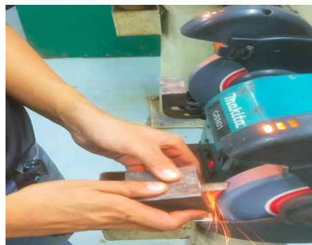
5. Grind the end relief angle using the tool bit jig.
