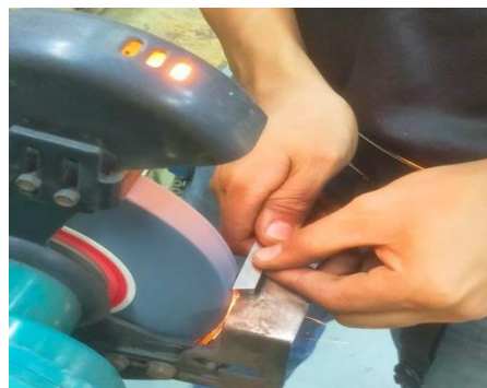
8. Grind the side rake using bare hands.
