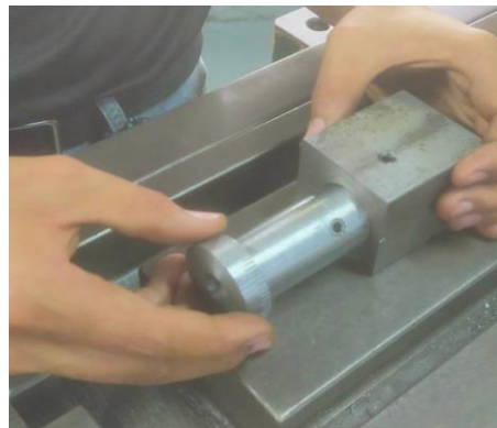
3. Put the sleeve inside the barrel
