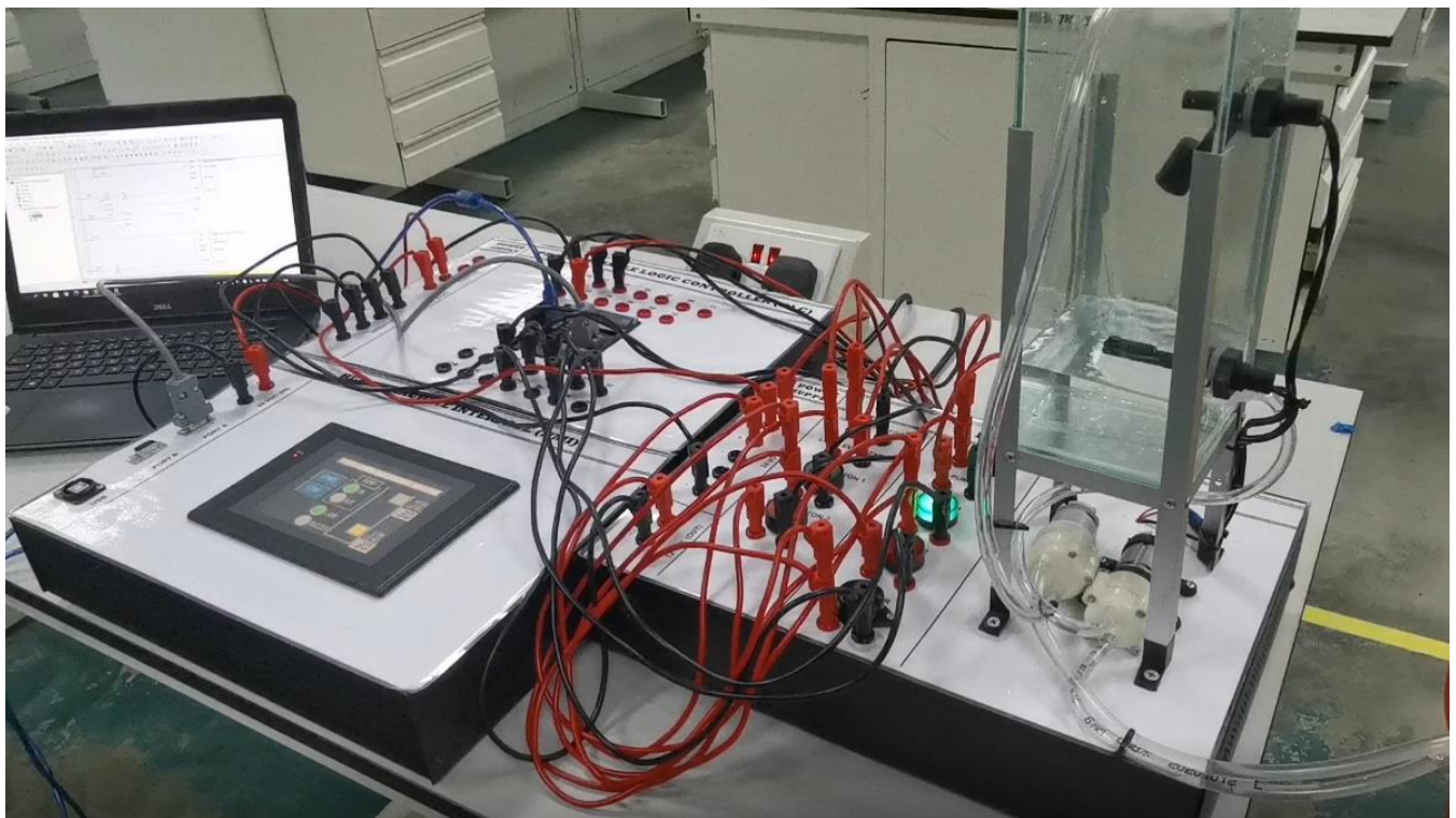
Figure 4 In & Out Water Control System Application Kit with PLC And HMI
