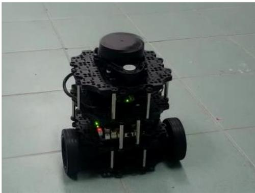
**Fig 5.** TurtleBot with LiDAR-based sensor
