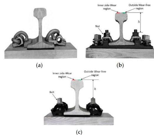
**Figure 3.** Rail fastener type: (a) Bolt-free fastener (b) nut-fastening fastener (c) bolt-fastening fastener [71].
