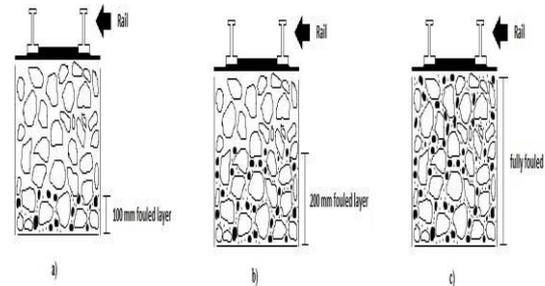
**Figure 2.** Ballast fouling condition a) 100 mm fouled layer b) 200 mm fouled layer c) fully fouled[61].
